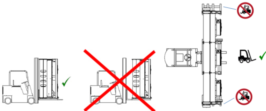
Figur 1. Correct lifting of Solar S/SR™ units with forklift
